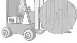
When unloading from a vehicle, use either the tail-lift / elevator or a suitable aid such as a forklift truck. Never let reels drop from the vehicle to the ground !
