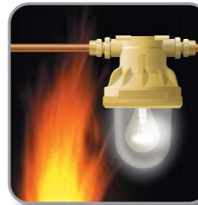
**FIRE RESISTANCE** – weaker situation is copper melting point (1082°C) MICO® is the safest cable, it can withstand to severe fire, water and mechanical tests as foreseen by British (LPCB), European and australian standards
