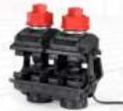
ATOM insulated Piercing Connector CBSpriCN 95 2p is used to achieve contact by simultaneously piercing the insulation on LV ABC conductors of main power distribution line and on LV ABC network connection conductor.
