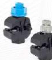
ATOM insulated piercing Connector CESpriCNT 95 is used to achieve contact by simultaneously piercing the insulation on LV ABC conductors of main power distribution line and on LV ABC conductors of street lighting connection line or other small electricity consumer.
