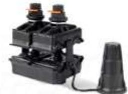
ATOM Connector insulated piercing connector is used to achieve contact by simultaneously piercing the insulation on LV ABC conductors of main power distribution line and on insulated copper or aluminum conductors of network connection lines.
